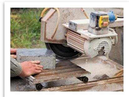
Most stationary saws come equipped with a water basin that typically holds several gallons of water and a pump for recycling water for wet cutting. Handheld saws spray water that is held in separate containers.
