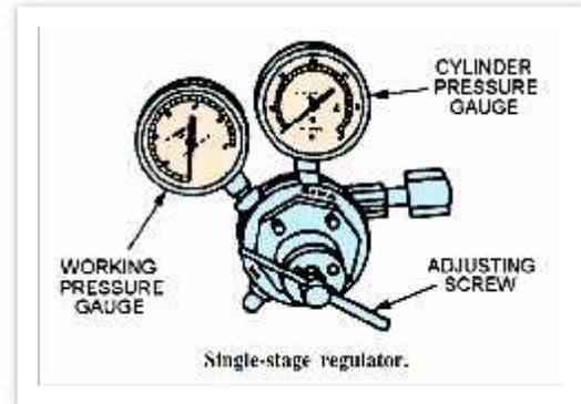
Acetylene regulators and oxygen regulators are of the same general type, although those designed for acetylene are not made to withstand such high pressures as are those designed for use with oxygen cylinders.
