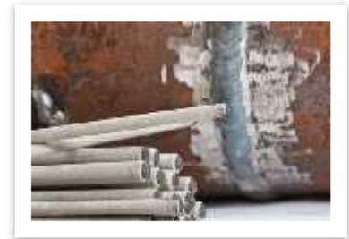
**Welding Rods:** The term welding rod refers to a filler metal, in wire or rod form, used in gas welding and brazing processes and in certain electric welding processes (tungsten inert gas) in which the filler metal is not a part of the electric circuit. A welding rod serves only one purpose—it supplies filler metal to the joint.
